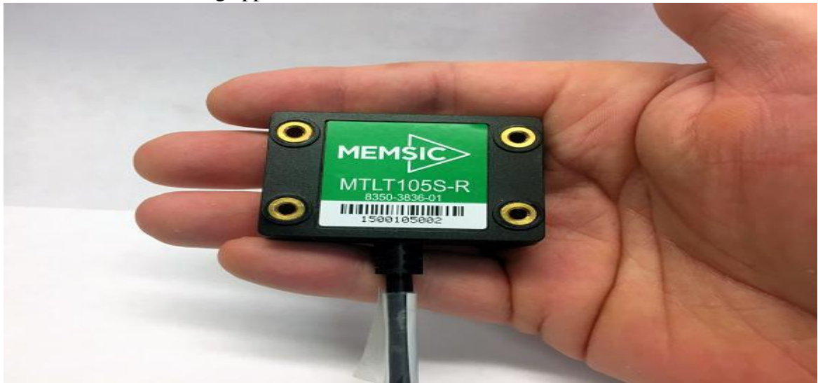
Fig :Incorporating both an accelerometer and a gyroscope, Tilt sensors help drones maintain level flight.
