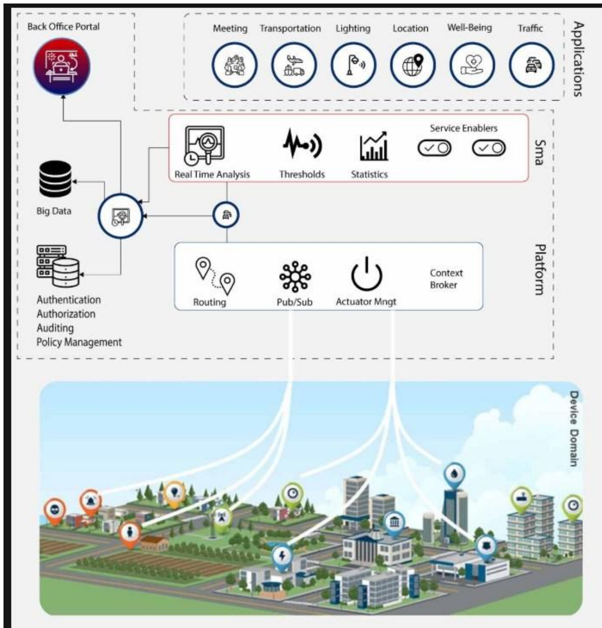
Figure 1: Smart City Architecture with IoT Devices
