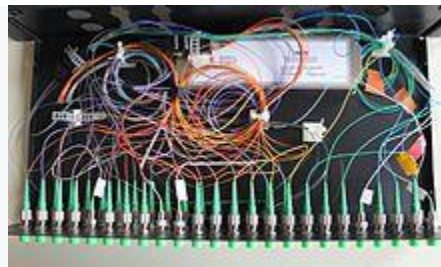
WDM multiplexer for DWDM communications
