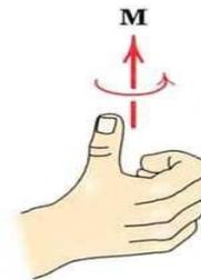
Sign consistency with in a given problem is very important. The moment  $M$  may be considered sliding vector with a line of action coinciding with the moment axis.
