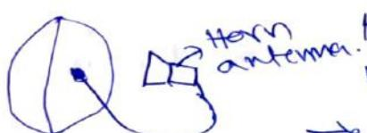
⇒ Waveguide Horn antenna is the primary radiator. which is pointing the parabolic antenna.
